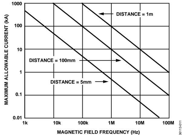
Figure 11. Maximum Allowable Current for Various Current-to-ADuM1250/ADuM1251 Spacings
