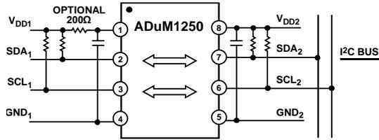
Figure 9. Typical Isolated I<sup>2</sup>C Interface Using the ADuM1250
