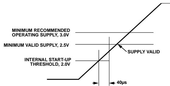
Figure 8. Start-Up Condition, Supply Slew Rate < 12.5 V/ms
