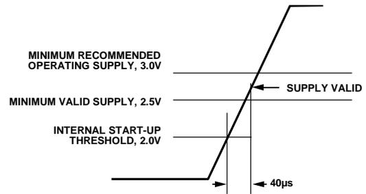
Figure 7. Start-Up Condition, Supply Slew Rate > 12.5 V/ms
