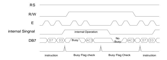
Example of 4-bit bus mode timing diagram
