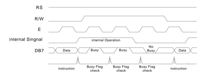
Example of 8-bit bus mode timing diagram
