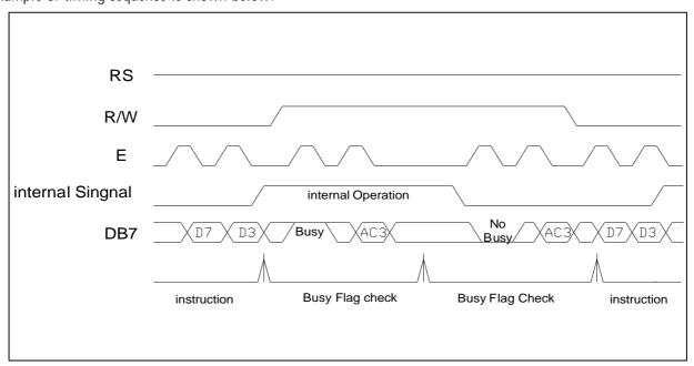
Example of 4-bit bus mode timing diagram
