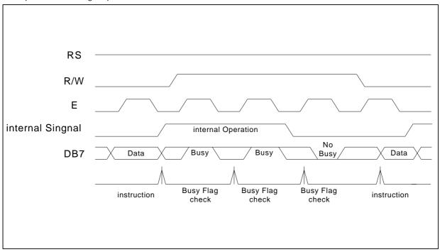
Example of 8-bit bus mode timing diagram
