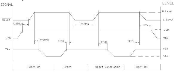
Please maintain the above sequence when turning on and off the power supply of the module. If VEE is supplied to the module while internal alternate signal for LCD driving (M) is unstable or RESET is active, DC component will be supplied to the LCD panel. This may cause damage to the LCD module.
