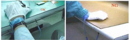
12.4 Please do not bend the film near the substrate glass.(this could cause film peeling and COF damage) and the peeling strength about 600g/cm, the bending <20times and the bending radius :R>0.8mm
