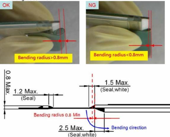
12.5 Avoid bending the film at IC bonding area.(>1.5mm)(this could damage the ILB bonding)
