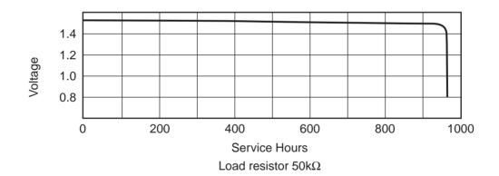
Average Service Capacity: 30 mAh (rated capacity at  $50k\Omega$  load, cut off voltage 1.2V at  $20^{\circ}C$ )
