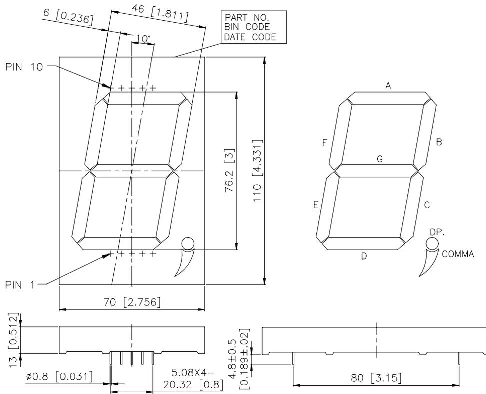
NOTES: All dimensions are in millimeters. Tolerances are  $\pm 0.25\text{mm}$  (0.01") unless otherwise noted.
