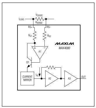
Figure 2. MAX4080 Functional Diagram
