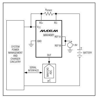
Figure 5. MAX4081 Used In Smart-Battery Application
