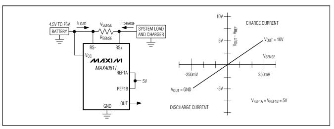
Figure 1. MAX4081T OUT Transfer Curve
