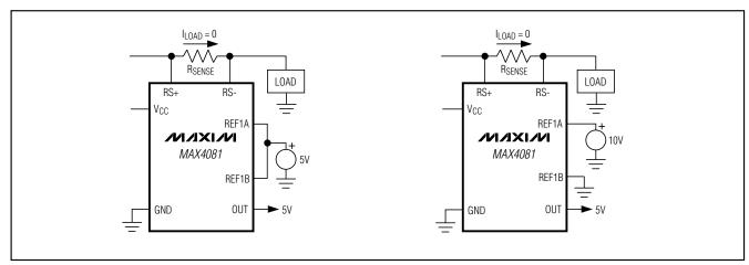
Figure 4. MAX4081 Reference Inputs
