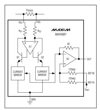
Figure 3. MAX4081 Functional Diagram
