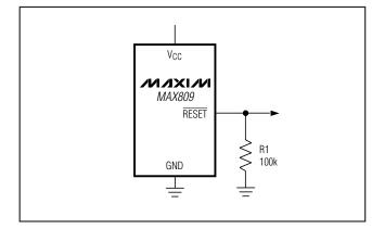
Figure 2. RESET Valid to Vcc = Ground Circuit
