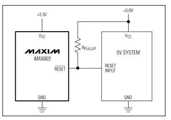
Figure 4. MAX803 Open-Drain RESET Output Allows Use with Multiple Supplies
