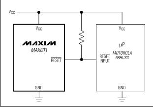
Figure 3. Interfacing to µPs with Bidirectional Reset I/O
