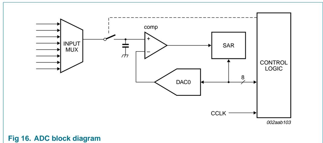
Fig 16. ADC block diagram
