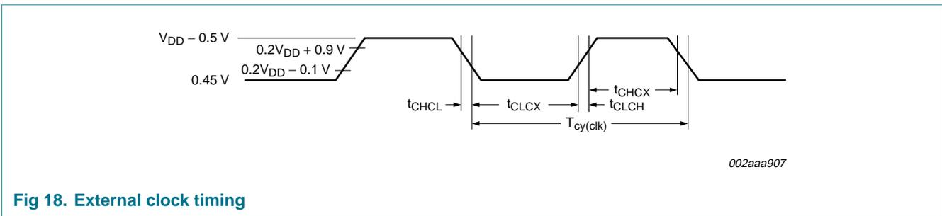
**Fig 18. External clock timing**
