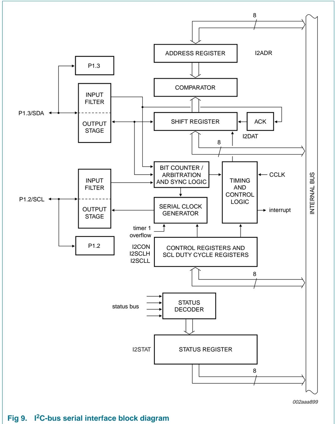
**Fig 9. I<sup>2</sup>C-bus serial interface block diagram**
