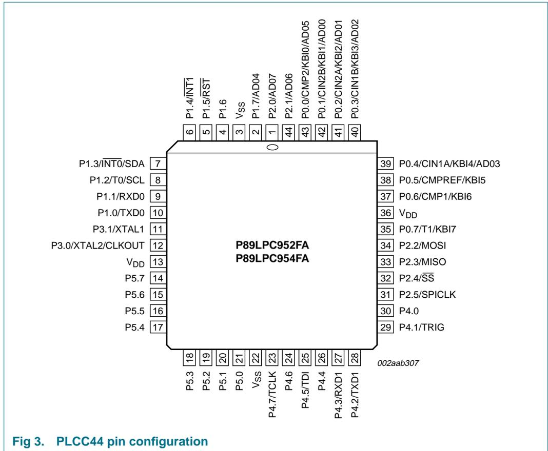
Fig 3. PLCC44 pin configuration
