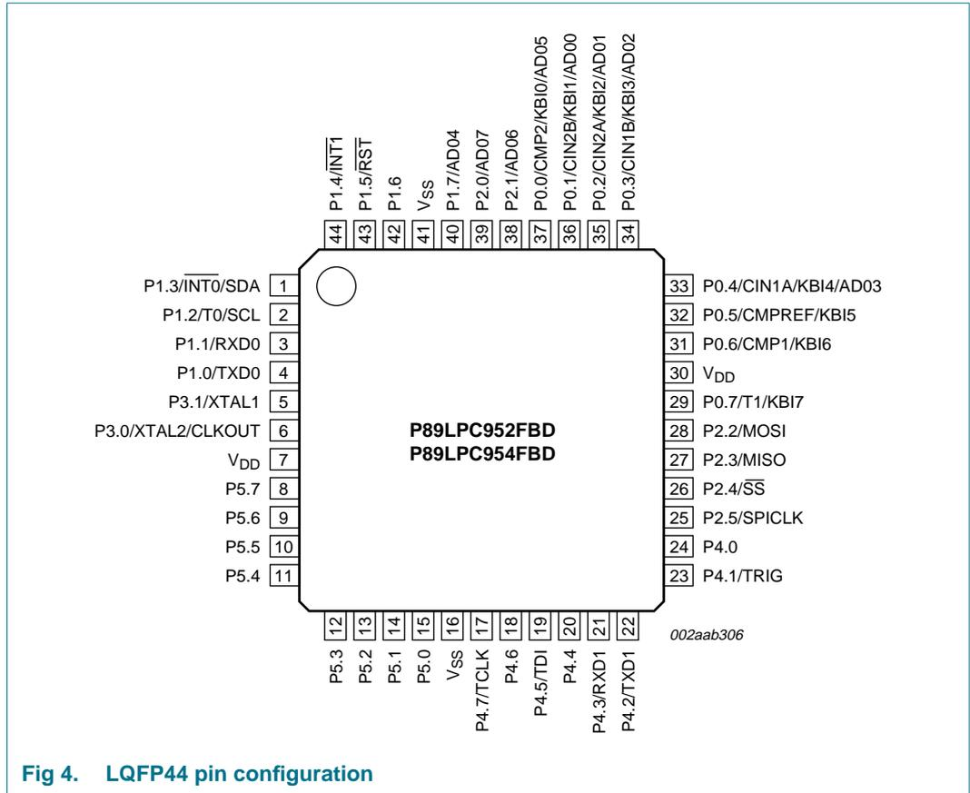
Fig 4. LQFP44 pin configuration
