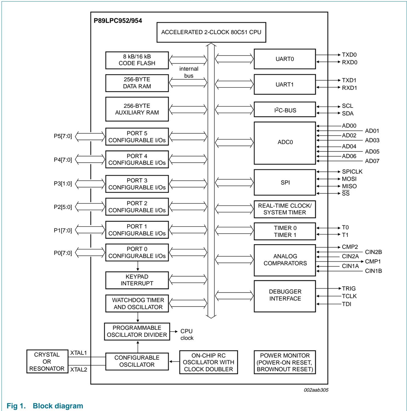
**Fig 1. Block diagram**
