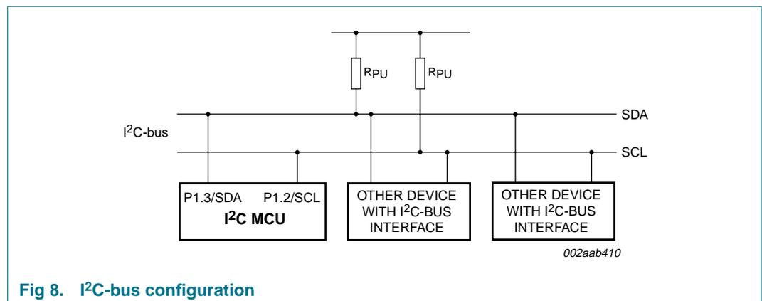
**Fig 8. I<sup>2</sup>C-bus configuration**
