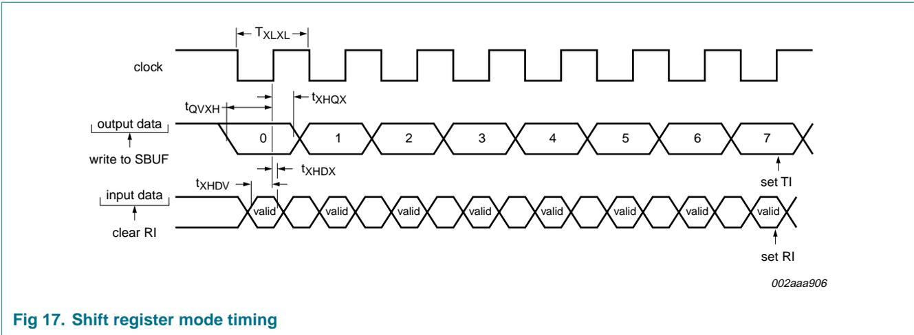
**Fig 17. Shift register mode timing**
