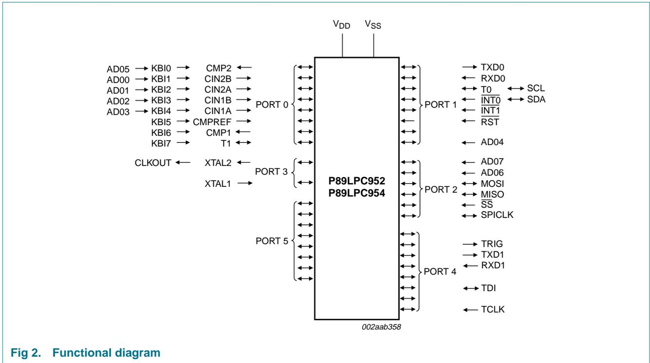
**Fig 2. Functional diagram**
