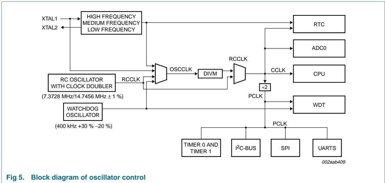
Fig 5. Block diagram of oscillator control
