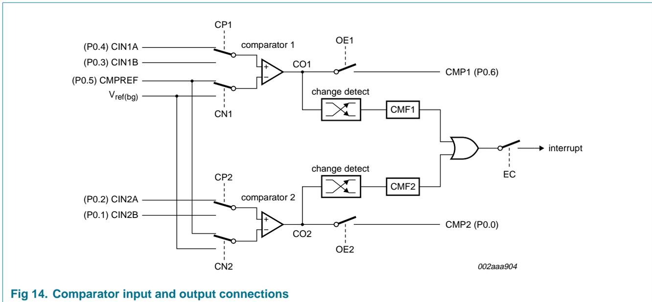
Fig 14. Comparator input and output connections
