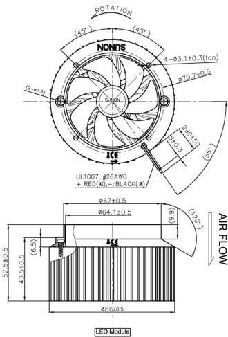
Assembly direction of customer's LED Module
