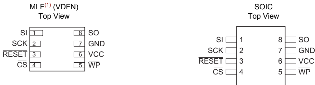
Figure 1-1. Pin configurations and pinouts.
