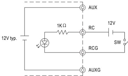
(B) Using internal 12V auxiliary output
