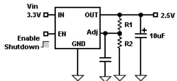
A capacitor from Adj to Ground provides greatly improved noise performance.
