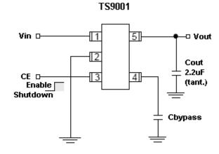
CE (pin 3) may be connected directly to Vin (pin 1) Low noise operation: Cbypass=470pF, Cout>2.2uF Basic operation: Cbypass=not used, Cout>1uF
