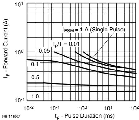
Figure 3. Pulse Forward Current vs. Pulse Duration
