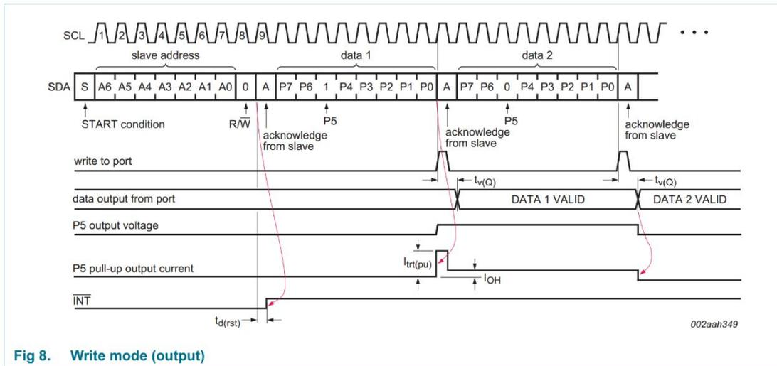
Fig 8. Write mode (output)
