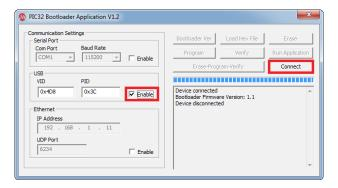
2. Press the **Load Hex File** button, select the update file, and after the file has been loaded, press the **Erase-Program-Verify button**.
