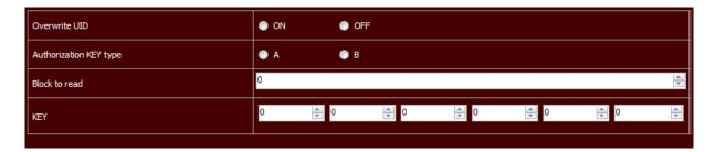
**Overwrite UID** – function that enables block reading. Enabling this option overwrites the UID code with the content of the card,
