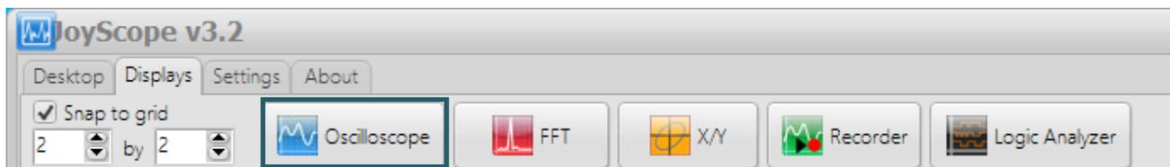
It may happen that you receive the message “Device not in analog mode”. In this case, you must open the JoyScope Mx50 control unit and switch the device to analog mode in **DAQ mode**.
