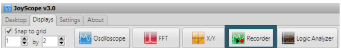
The standard oscilloscope window opens and offers you the **Recorder** button, by which you can use to start recording the measurement data.
