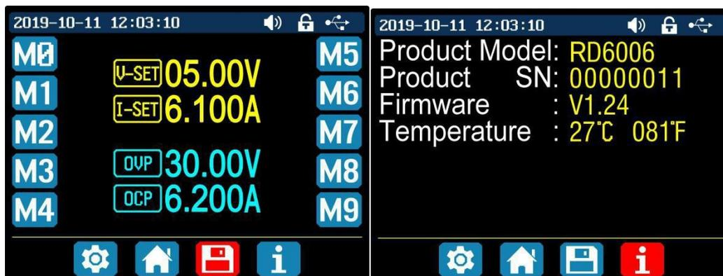
You can press '**SHIFT**' + '**MENU**' to enter the system setting menu, and then press the right button three times to enter the system information menu as shown above. You can view the SN number, firmware version and system temperature here.
