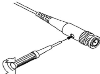
**Probe Attenuation Setting:** Probes are of various attenuation factors which affect the vertical scale of the signal. The Probe Check function is used to verify if the Probe attenuation option matches the attenuation of the probe.
