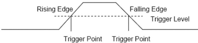
**Slope:** Select the trigger slope to rising, falling, rising & falling.
