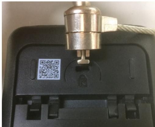
A safety keyhole is reserved on the back shell of the oscilloscope. Users need to purchase the safety lock by themselves. Wrap one end of the safety lock around a hard-to-move object, insert the other end into the safety lock hole, turn the key clockwise to lock the instrument, and then pull out the key. In this way, the most basic anti-theft requirements can be achieved.
