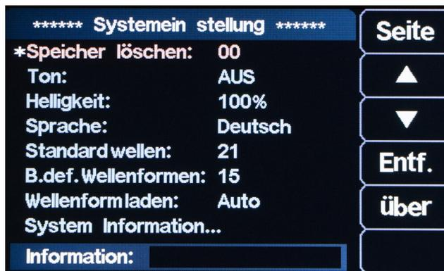
Press the **SYS** menu button to enter the system settings and press ▲ ▼ to select items such as Clear Memory, Sound, Brightness, Language, Built-in Wave Count, arb Wave Count, Waveform Load, Methods, System Information, etc.
