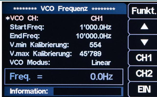
VCO stands for voltage-controlled oscillator. A voltage-controlled oscillator is an electrical oscillator whose frequency can be changed by the magnitude of an applied voltage. Press **VCO** and the **FUNC** menu key to select the frequency control, amplitude control and duty cycle control functions.
