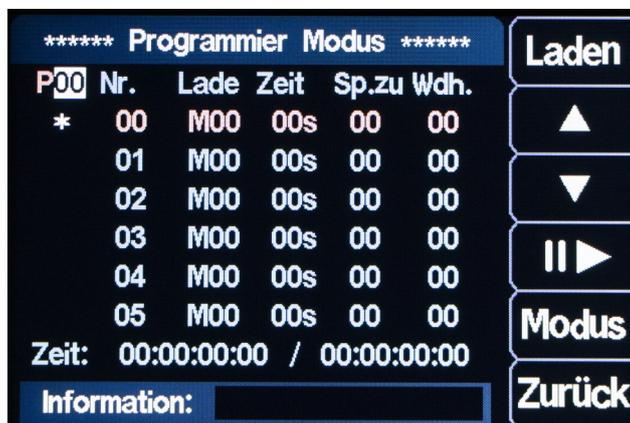
Programming mode allows a sequence of different signals to be output automatically. Press **FUNC** to enter the programming mode menu and the MODE menu key to switch between normal mode and debug mode.
