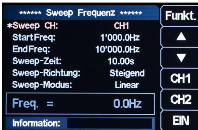
With the sweep function, a start and end value can be set, the set range is swept through in the set time. This can be used for frequency, amplitude and duty cycle.
