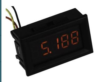
The VM533 digital voltmeter can precisely measure voltages of up to 33V and display them on the integrated 0.36" 5-digit segment display.
