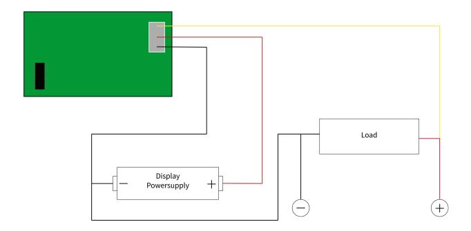
The provided plug of the digital voltmeter has 3 cables.
