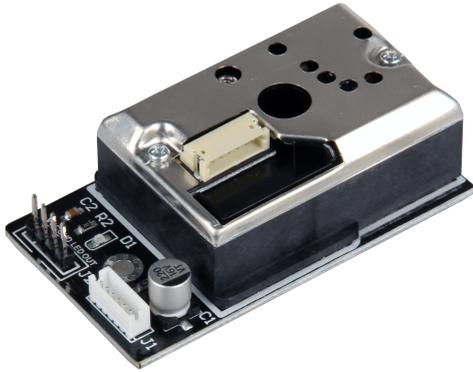
The GP2Y1014AU is an optical sensor for the detection of dust particles.
