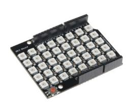
The LEDs are connected in a continuous series. Each LED can be individually receive a color value by digital control. This makes it possible to generate complex color light shows. Each LED can display up to 16 million colors (256 brightness levels/color).
