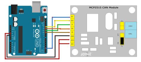
If you are using an Arduino Mega, please note that the SPI interface is connected to different pins than the Arduino UNO.
