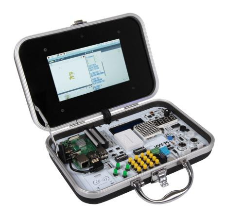
With the Joy-Pi, Joy-iT has developed a comprehensive education solution and applied its many years of experience in the production of open source electronics. The Joy-Pi is an experimental case based on the Raspberry Pi and is ideal for the entry into electrical engineering and programming.
