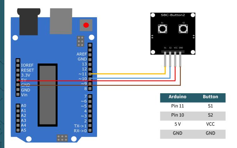
The following example program displays the status of the two buttons every 2 seconds.
