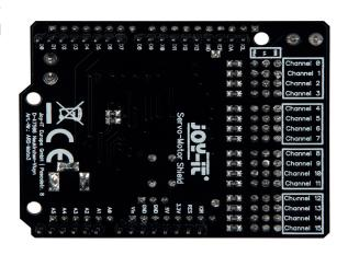
Your power supply must be adjusted of its performance at your connected motors because insufficiently dimensioned power supplies can be regonized that the motors are jerking instead of a flowing movement. We recommend the application of our 4.8A power supply which offers a continuous output of 24W.
