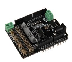
The Motorino board is an extension-board to control and use up to 16 PWM-controlled 5V-Servo-motors. The control and the programming can be done, as usual, with the Arduino.
