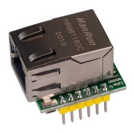
With this SPI-Ethernet interface converter you can expand for example your Arduino or your Raspberry Pi Pico with an Ethernet interface.
