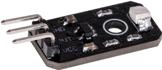
The analog GUVA-S12SD UV sensor is a UV-A and UV-B sensitive photodiode and detects the intensity of the ultraviolet radiation affecting it. The detection range covers rays with a wavelength of 240 - 370 nm.
