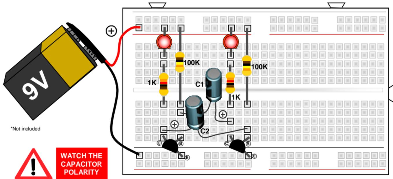
**Required parts:** 9V battery\*, 2x 1K resistor (brown black red gold), 2x 100K resistor (brown black yellow gold), 2x red LED, 2 x BC547 transistors, 2x 10 $\mu$ F electrolytic capacitors
