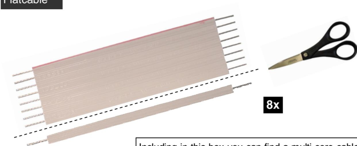
Including in this box you can find a multi-core cable. The wires must be separated from each other before use. This can be done using a wire-cutter or pair of scissors. Use the separate wires to connect components (indicated in the drawing by a thick black line) Velleman part# FC8)
