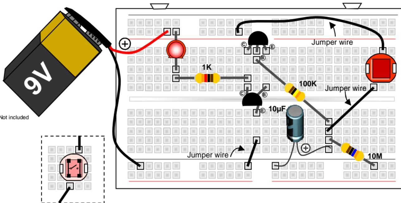
**Required parts:** 9V battery\*, 1K resistor (brown black red gold), 100K resistor (brown black orange gold), 1M resistor (brown black green gold), Red LED, push-button, 2x BC547 transistor, 10 $\mu$ F electrolytic capacitor, 3 x wire jumper
