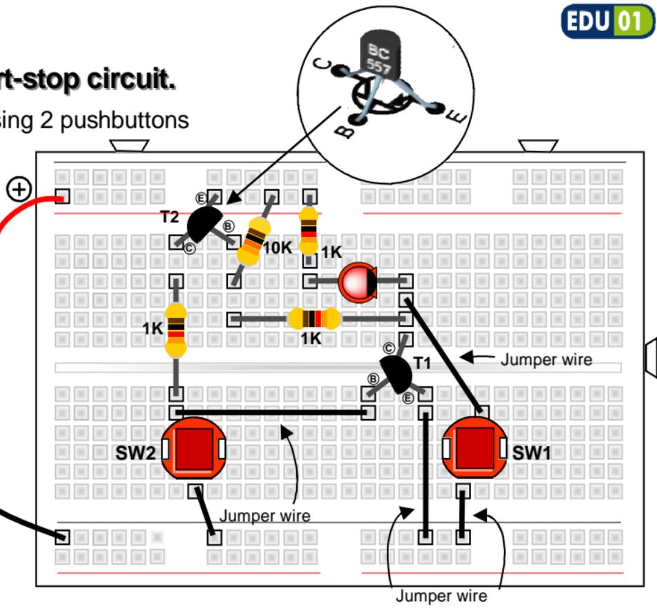
**Required parts:** 9V battery\*, 3 x 1K resistor (brown black red gold), 10K resistor (brown black orange gold), red LED, 2 x push-button, 1x BC547 transistor, 1x BC557 transistor, 5 x wire jumper
