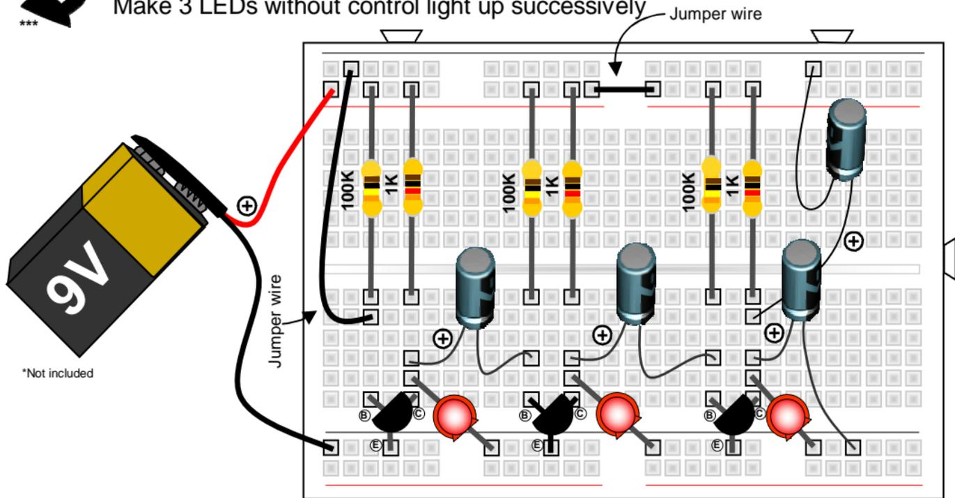
**Required parts:** 9V battery\*, 3x1K resistor (brown black red gold), 3x100K resistor (brown black yellow gold), 3 x red LED, 3x BC547 transistor, 3x10 $\mu$ F electrolytic capacitor, 2x wire jumper
