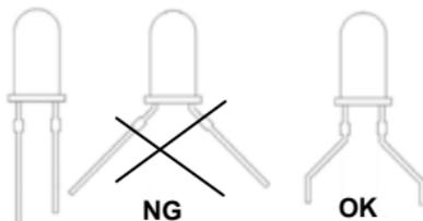
A LED is a **Light Emitting Diode**, it can emit light using a small current (max 20mA with a 1.8V drop).
