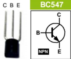
A transistor is an amplification device. By means of a small current, a much larger current is controlled. Transistors come in two flavours, NPN and PNP-types, depending on the polarity. With this kit, you receive a BC557 (PNP) and a BC547 (NPN) transistor. A transistor has 3 pins: Base, Emitter and Collector. (Velleman part# BC557B, BC547B)
