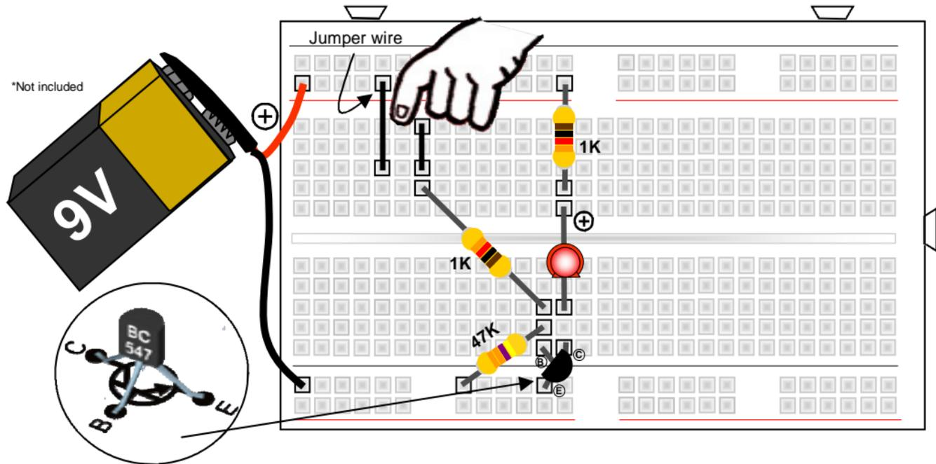
**Required parts:** 9V battery\*, 1K resistor (brown black red gold), 470K resistor (yellow purple yellow gold), red LED, BC547 transistor, wire jumper.
