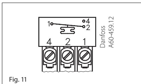
KPS temperature controls are fitted with a Pg 13.5 screwed cable entry suitable for cables from 5 – 14 mm. Contact function is shown in fig. 11
