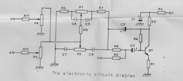
As you can see the circuit has an input for the signal and two outputs which can be used to split the signal between two different appliances, (i.e. two line amplifiers, a monitor amplifier and a small amplifier etc.) Connected as it is shown in the diagram a 1126 with a 1127 form a complete compact microphone preamplifier with tone controls and master volume.
