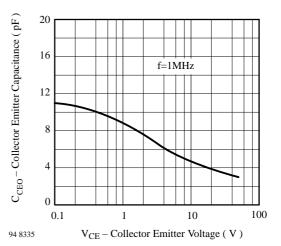
Figure 6. Collector Emitter Capacitance vs. Collector Emitter Voltage
