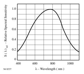
Figure 8. Relative Spectral Sensitivity vs. Wavelength
